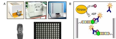
**Fig. 1. A.** PamStation®4, 12 and 96 instruments and PamChip®4 and PamChip®96 array plates used for kinase activity profiling. **B.** The reaction takes place on spotted peptides on the array. Peptide phosphorylation through active kinases, or inhibition thereof, can be monitored in lysates of cell lines or tumor tissues by real time fluorescent readout, using a fluorescently labeled phospho-tyrosine specific antibody
