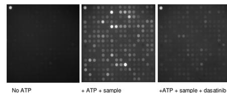
**Fig. 2.** Images of PamChip® arrays after incubation of the array with a cell lysate in the absence (left) and presence (middle) of ATP and the effect of addition of the inhibitor dasatinib to the incubation mixture (right).
