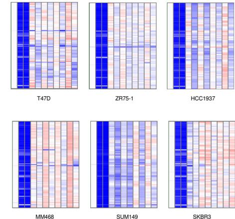
**Fig 6.** The effect of five inhibitors on peptide phosphorylation for 6 cell lines. Inhibitors from left to right for each cell line: no inhibitor, 0.5 and 5 µM of dasatinib, erlotinib, gefitinib, imatinib and lapatinib. Signals are normalized to the control without inhibitor.
